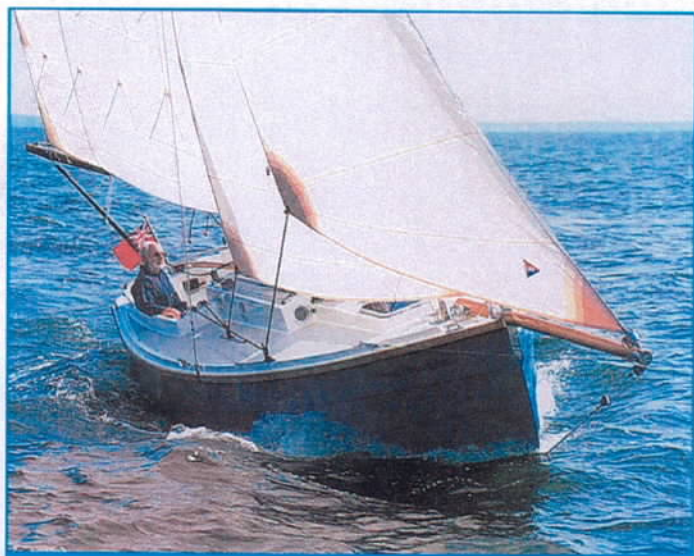
D ripping with old-fashioned charm, the Crabber 22 has modern conveniences like roller furling and a 9-horsepower inboard diesel, and it can be easily trailered.
