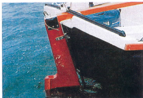
The mechanism on the rudder to raise and lower a small lifting plate for more bite on the water
