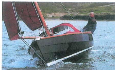
Multi-chined effect disguises the glassfibre hull
