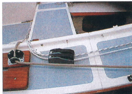
Main halyard and lazyjack/topping lift are led through clutches on the side-deck
