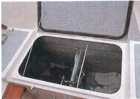
The drum for raising and lowering the steel centreplate is housed in the midships locker
