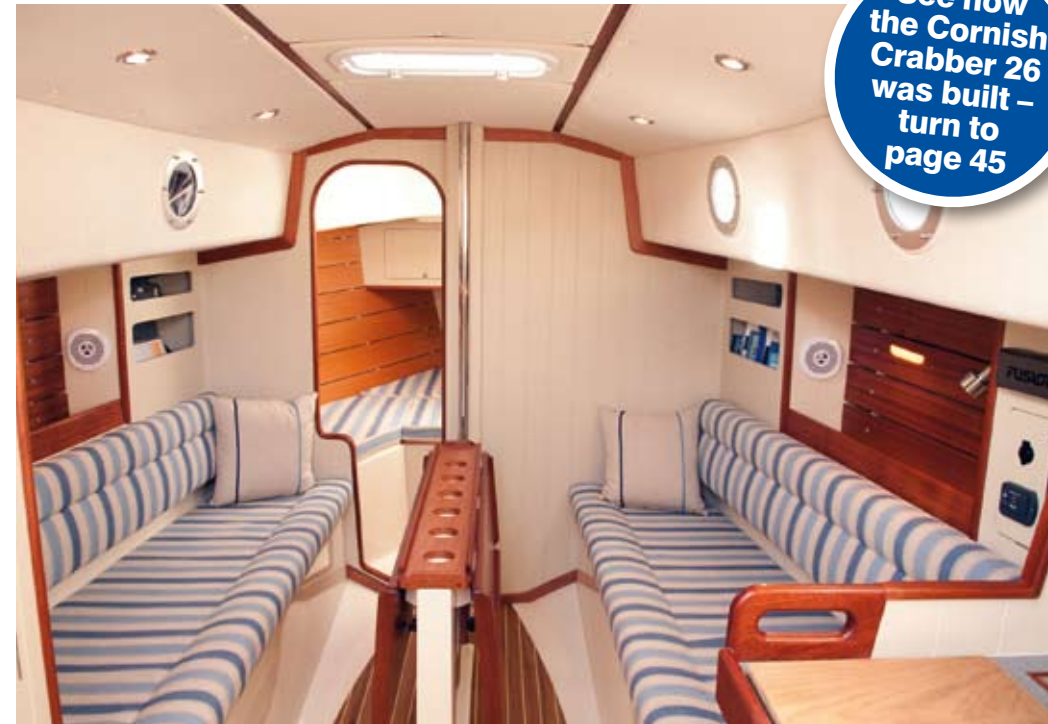
The Crabber's saloon is bigger than on many larger boats because there's no aft cabin to push the companionway forward. A door to close off the forecabin would be impractical, so a simple curtain does the job
