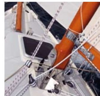
A tabernacle allows the mast to be raised and lowered afloat
