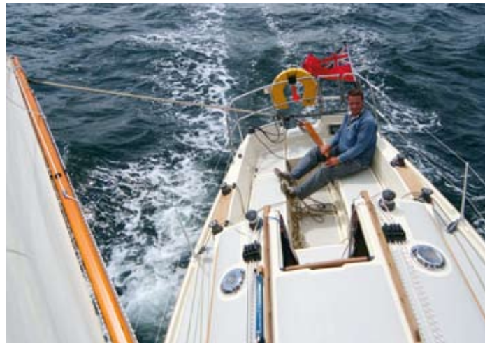
The deep and well-protected cockpit is a good leg-bracing width between the seats. Deck hardware includes vents over the galley and heads
