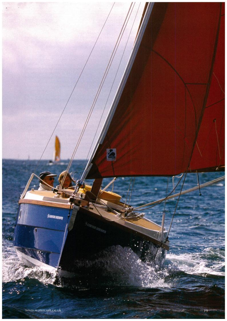
the wide coachroof is very good, so there is no difficulty getting forward to the little, sunken foredeck for anchoring or mooring. The little bowsprit runs over the foredeck, from the wooden housing forward of the cabin and through a gammon iron on the stem. This is stainless steel, like the mast tabernacle, the other deck fittings and the rigging.
