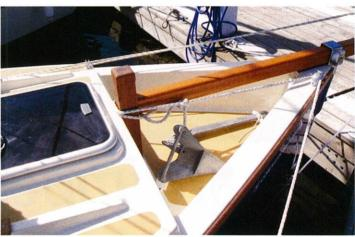
coachroof to provide a permanent, non-slip surface, as well as for the cockpit floor, which is raised to allow it to self-drain. Ballast punchings are resined into her bilges just under the cabin sole and there are two buoyancy compartments built into the aft ends of the cockpit seats. Her construction is simple and strong and low maintenance, just what is needed if your leisure time is limited and you'd rather be sailing.
